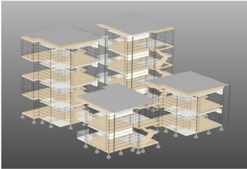
Figure 5: Ground Slab, Suspended Slab and Roof
